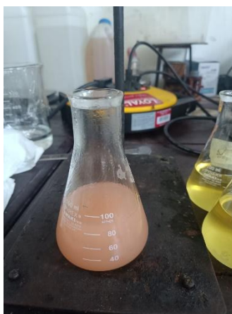
Figure 6. Free Fatty Acid measurement of used cooking oil.
