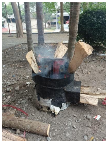
Figure 9. Carbonization process with slow pyrolysis at 300°C for 3-4 hours using biomass stove.
