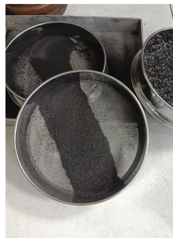
Figure 11. Sieving process of fine cocoa bean charcoal using 40, 60, and 100 mesh.
