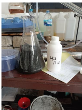
Figure 12. Soaking cocoa bean shell charcoal with 1 liter 10 M HCl.
