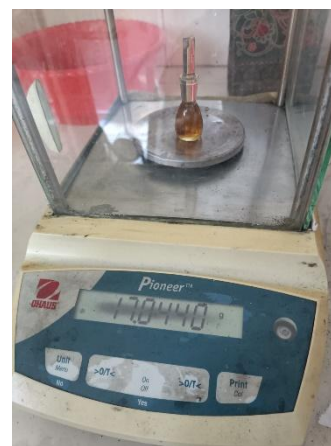
Figure 7. Density measurement using pycnometer method.
