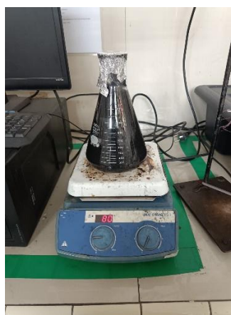
Figure 13. Mix, stir, and heat cocoa bean shell charcoal + HCl on a hot plate.
