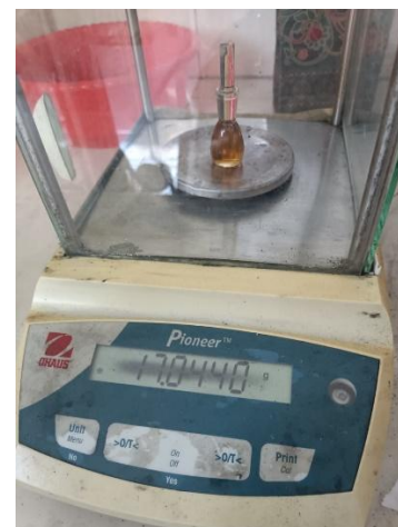
Figure 20. The density test of used cooking oil after the adsorption process.
