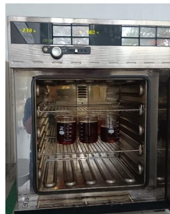
Figure 4. Water content removal using oven at 105-110°C for \pm 1 hour.
