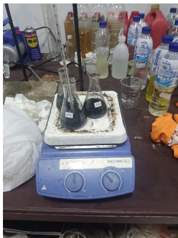
Figure 16. The process of adsorption of FFA levels using cocoa bean husk by heating and stirring.
