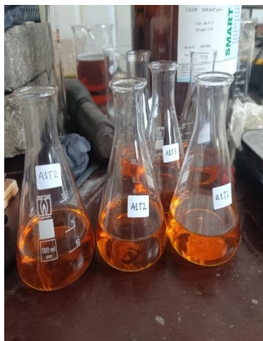
Figure 15. Taking 50 ml of used cooking oil for the FFA level reduction test process.
