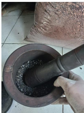
Figure 10. Grinding process of cocoa bean husks charcoal using mortar and pestle.
