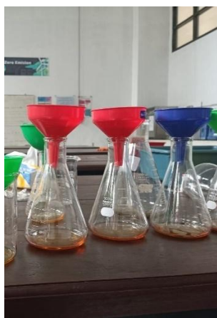
Figure 5. Insoluble impurities removal using filter paper.
