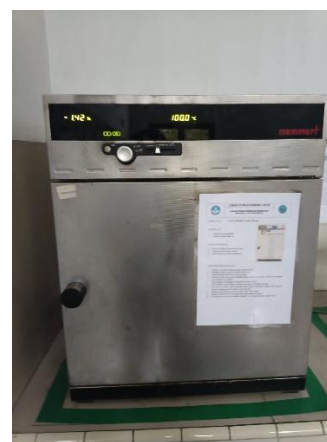
Figure 14. Heat the cocoa bean husks charcoal in the oven at 110°C for \pm 3 hours.
