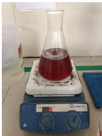
Figure 3. Homogenized 1.5 liters used cooking oil with magnetic stirrer on 500 rpm
