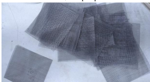
Gambar 3. Substrat stainless steel mesh (304 woven wire mesh 50)
